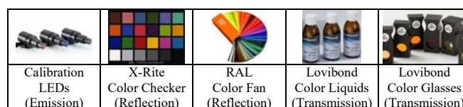
Fig. 03. Calibration standards for color inspections and measurements
